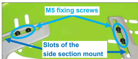
Figure 64: M5 fixing screws and elongated holes of the side section mounts (SPEEDY 4all Ergo and -4you Ergo)
