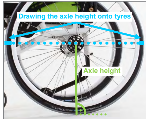
Figure 79: Drawing the axle height on the front and back of both tyres
