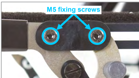
Figure 154: M5 fixing screws on the brake holding rail
