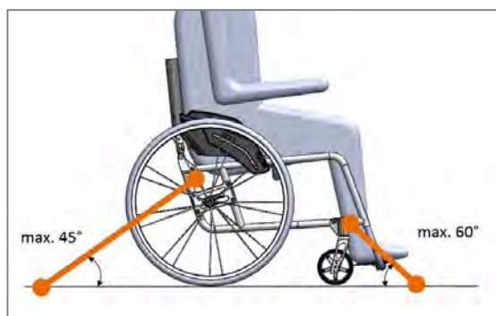
Figure 213: Run of the retractors at the front and rear with maximum tensioning angle and connecting points (view from the side)
