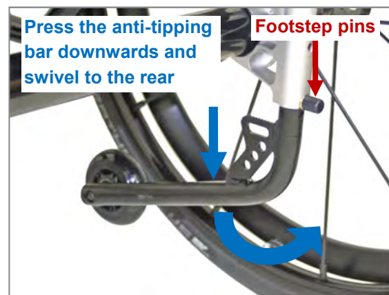
Figure 140: Moving the anti-tipping support to operating position (view from the rear)
