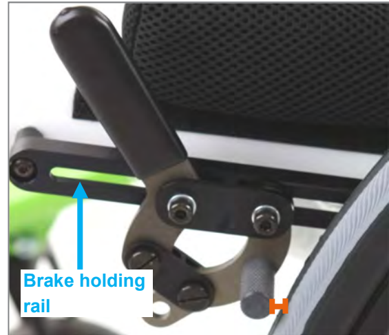
Figure 155: Distance between the brake pin and tyre of from approx. 3 to max. 4 mm with the brake opened
