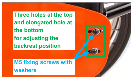
Figure 17: Adjusting the backrest position using holes in the side section
