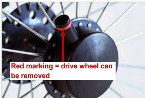
Figure 78: Tetra Clip with opened quick release axle, drive wheel can be removed
