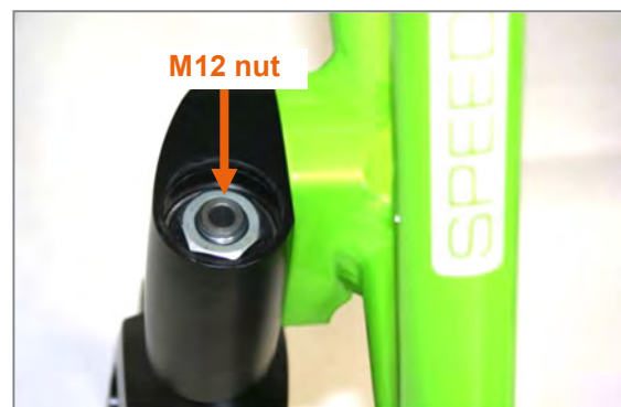
Figure 104: Aluminium cap removed and M12 nut visible
