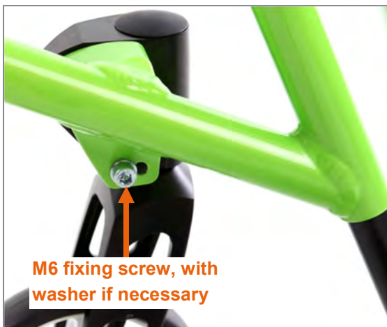
Figure 108: M6 fixing screw on frame inner side, washer fitted with G-shape frames but not V-shape frames
