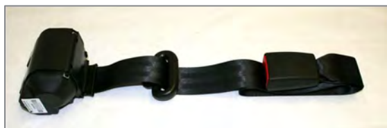
Figure 201: Automatic diagonal shoulder belt with deflector and buckle
