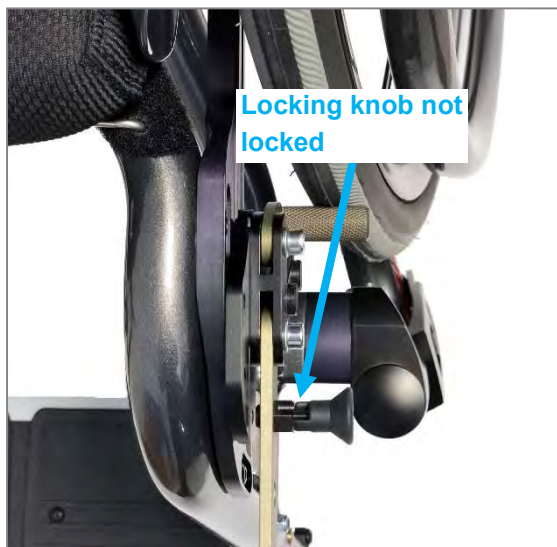
Figure 176: Locking knob pulled out of lock and turned 90°
