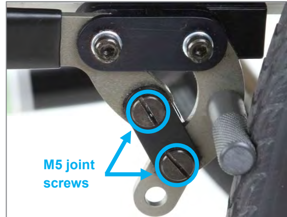
Figure 160: M5 joint screws for setting the actuating force of the brake lever
