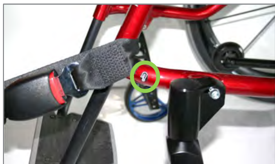
Figure 209: Symbol for front fastening and wheelchair loop at the front (example for SPEEDY 4you Ergo)
