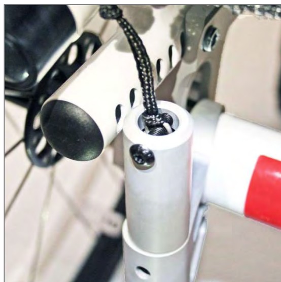
Figure 147: The M5 fixing screw screwed through the end eyelets of the tension spring
