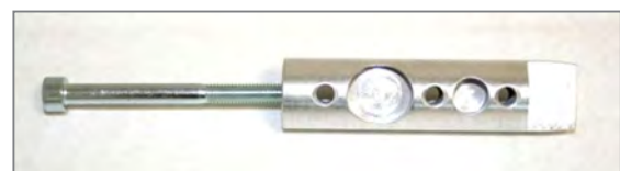
Figure 15: Short inlet with M6 screw screwed in (outside the frame for better illustration)
