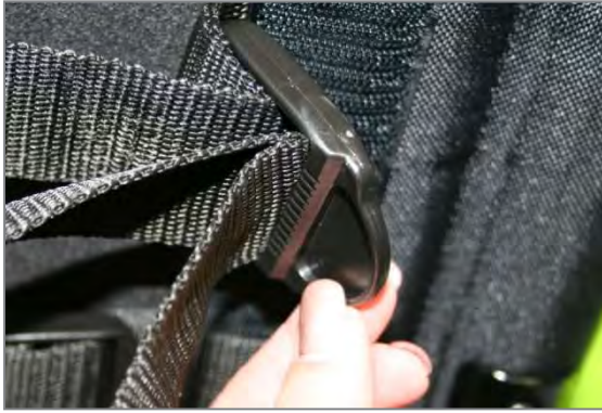
Figure 34: Step 5: Returning the belt through the tensioning loop to obtain the required "double passage"
