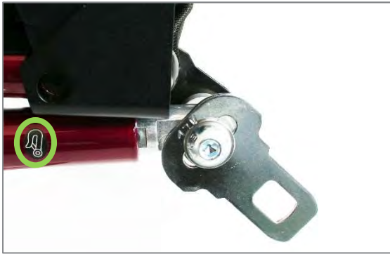
Figure 204: Transport restraint system attachment on the rear frame with latch plates for rear retractor and lap belt (view from the side)
