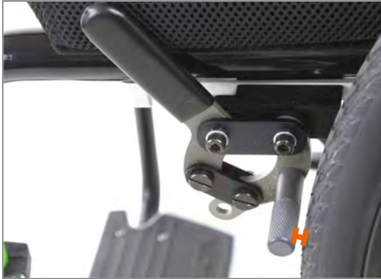
Figure 159: Distance between brake pin and tyre of approx. 3 mm to maximum 4 mm, with opened brake
