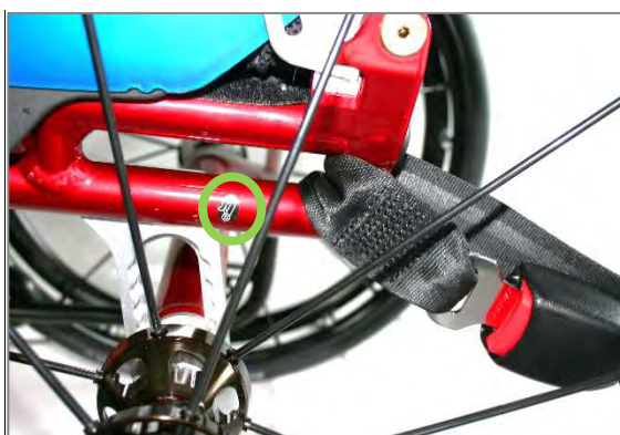
Figure 210: Symbol for rear fastening and wheelchair loop at the rear (example for SPEEDY 4you Ergo)
