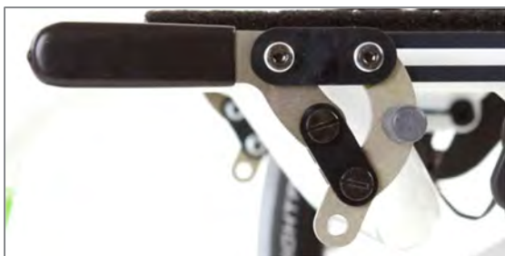
Figure 151: Knee lever brake system with standard brake lever
