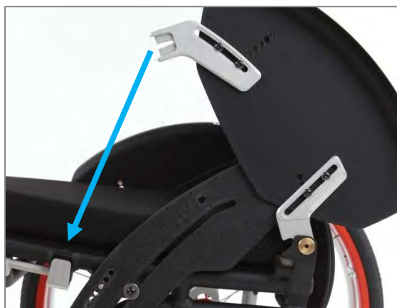
Figure 61: Rear side section mount mounted on back joint shaft (view without drive wheel)
