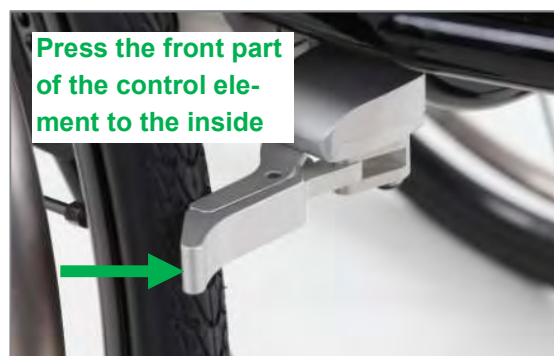
Figure 165: Integral brake closed, the brake is opened by pressing the control element towards the middle of the wheelchair
