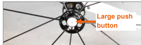
Figure 76: Quick-release axle with operation support, large push button
