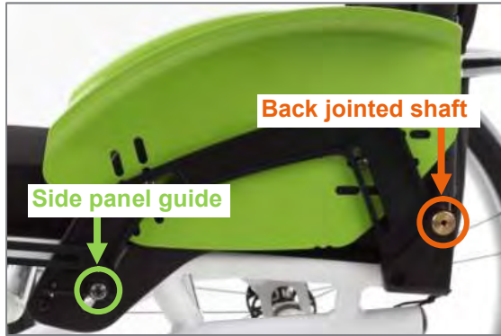
Figure 49: Clothing guard mounted on product (view without drive wheel)
