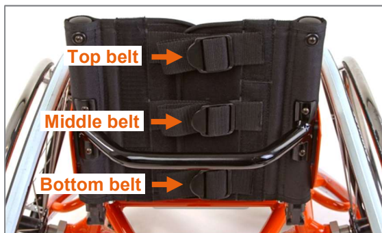
Figure 8: Belt system of the adaptable backrest upholstery with three belts
