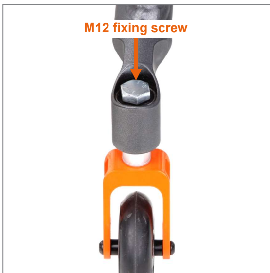
Figure 66: Cap removed and M12 fixing screw visible
