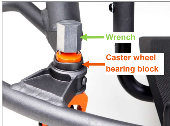
Figure 46: Loosen the nut of the caster wheel axle using the wrench
