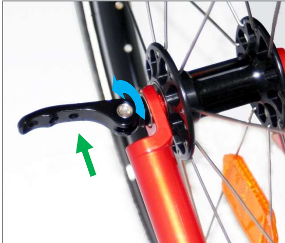
Figure 7: Open and turn quick release lever
