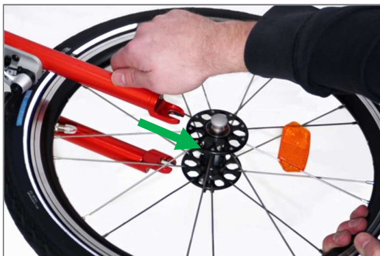
Figure 8: Remove the wheel by pulling downwards
