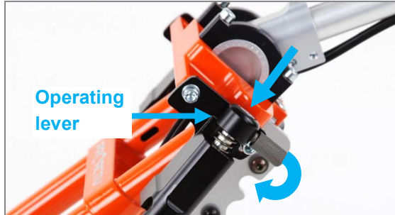
Figure 16: Press down and turn the operating lever
