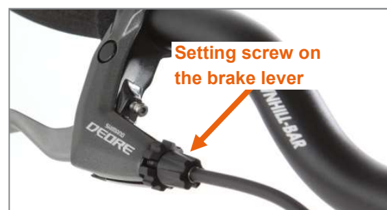
Figure 2: Setting screw on the brake lever
