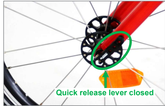
Figure 9: Quick release lever, tightened hand tight and closed
