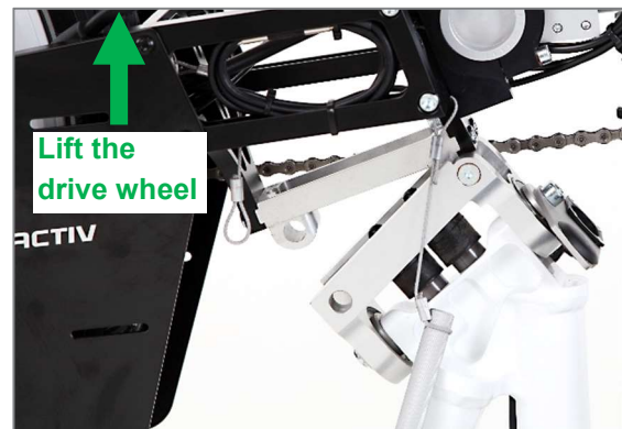
Figure 70: Lifting the drive wheel
