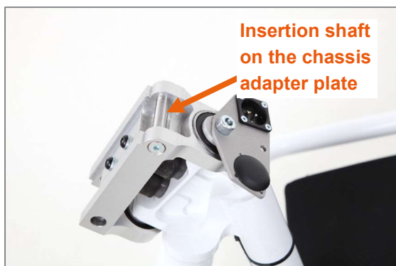
Figure 58: Insertion shaft on the chassis adapter plate
