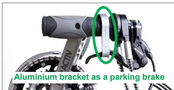
Figure 24: Aluminium bracket as a parking brake
