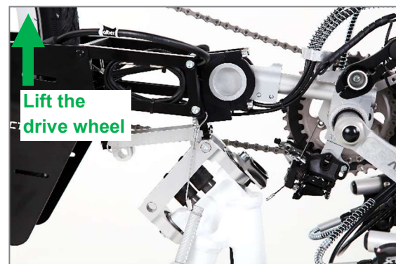
Figure 60: Lifting the drive wheel
