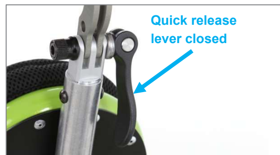
Figure 42: Quick release lever closed (view from behind)
