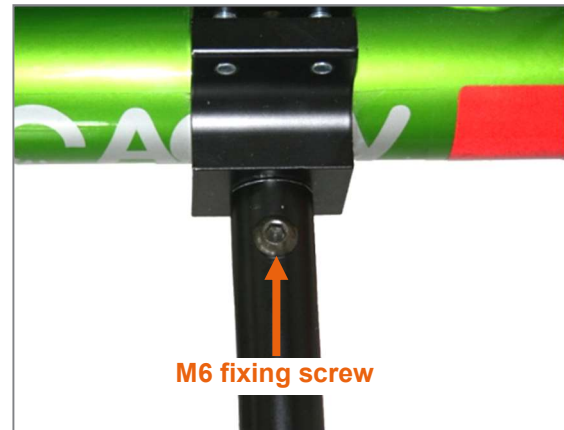
Figure 46: M6 fixing screws on the clamp on the axle tube
