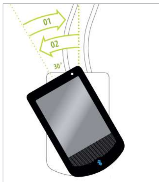
Figure 29: Attaching and removing the display
