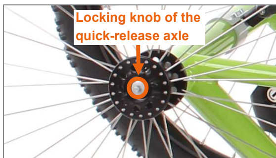
Figure 48: Locking knob of the quick-release axle in the middle of the wheel axle
