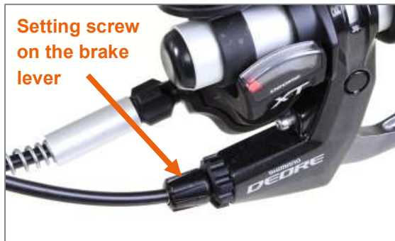
Figure 23: Setting screw on the brake lever
