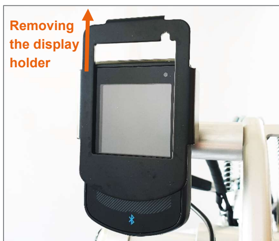
Figure 31: removing the display holder
