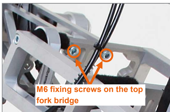
Figure 5: M6 fixing screws on the top fork bridge
