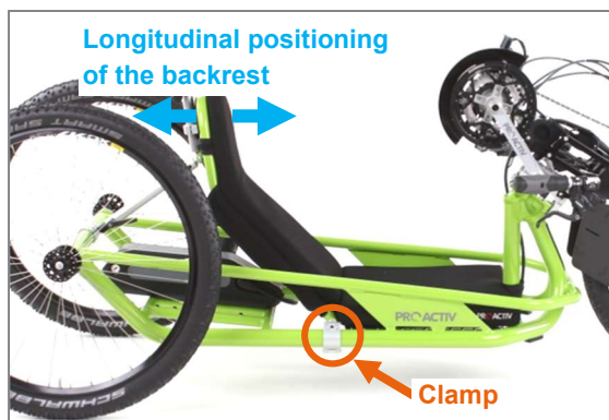
Figure 37: Clamp for the longitudinal positioning of the backrest
