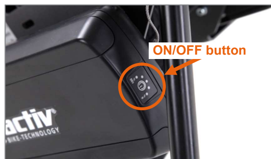
Figure 28: On and off button on the rechargeable battery
