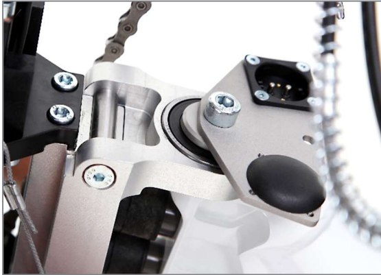
Figure 61: Insertion maul of the drive unit slips under the insertion shaft on the chassis
