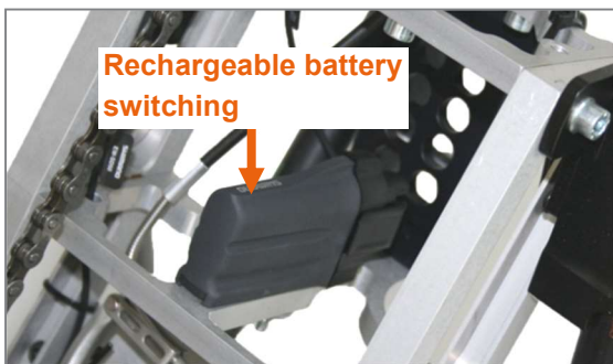
Figure 15: Alfine Di2 electronic gearshift battery
