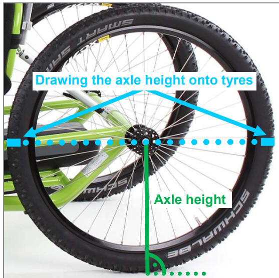
Figure 50: Drawing the axle height on the front and back of both tyres of the running wheels
