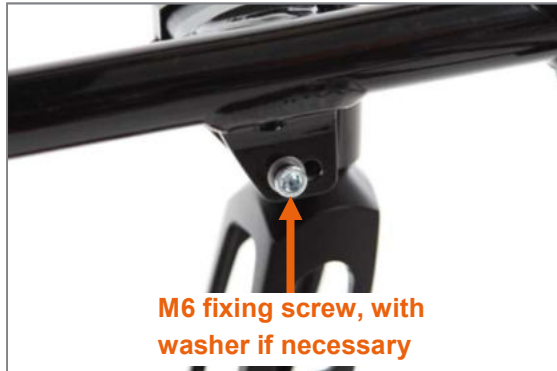
Figure 92: M6 fixing screw on frame inner side, washer fitted with G-shape frames but not V-shape frames
