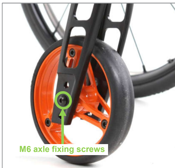
Figure 78: M6 axle fixing screw of caster wheel axle (view from outer side of product)
