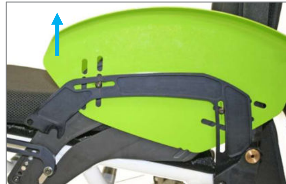
Figure 55: Clothing guard pulled from the side panel guide to the front (shown without drive wheel)
