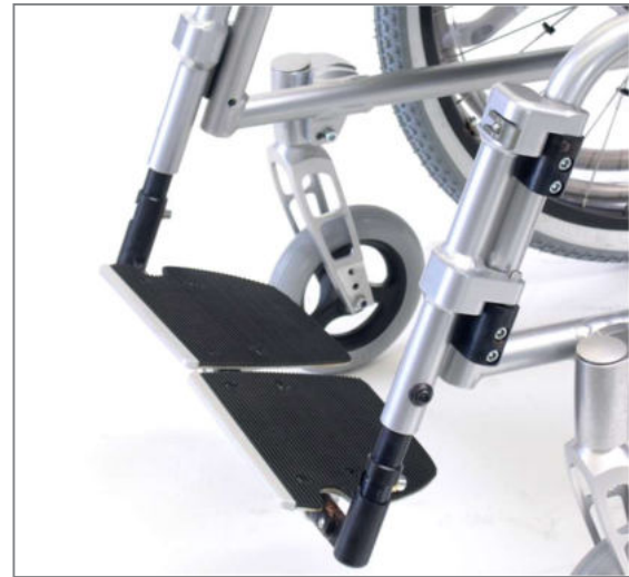
Figure 115: Swing away footrest, standard position
