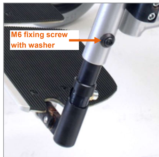
Figure 119: M6 fixing screw with washer to adjust the lower leg length
