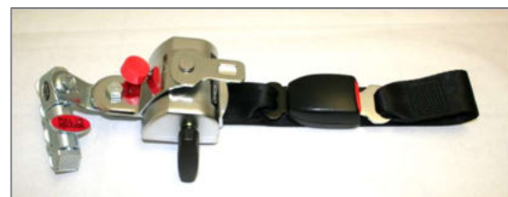
Figure 149: Rear retractor "semi-automatic" with hand wheel, buckle and belt link
