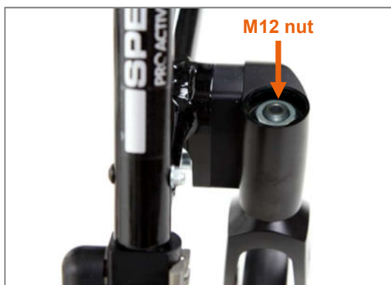
Figure 88: Aluminium cap removed and M12 nut visible
