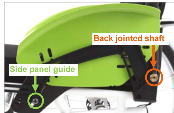
Figure 50: Clothing guard mounted on product (view without drive wheel)
