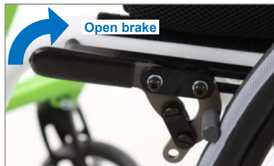
Figure 133: Brake closed; opening done by pulling the brake lever up and rearwards
