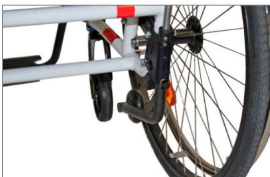
Figure 122: Passive position of anti-tipping support (view from the rear)
