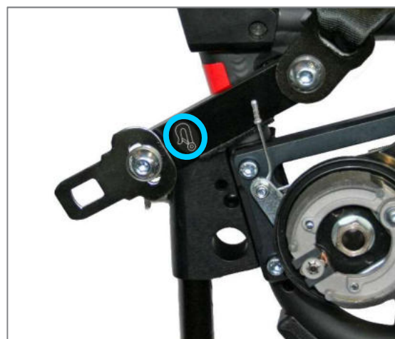
Figure 154: Transport restraint system attachment on the rear frame with belt link for rear retractor and lap belt
