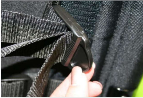
Figure 36: Step 5: Returning the belt through the tensioning loop to obtain the required "double passage"
