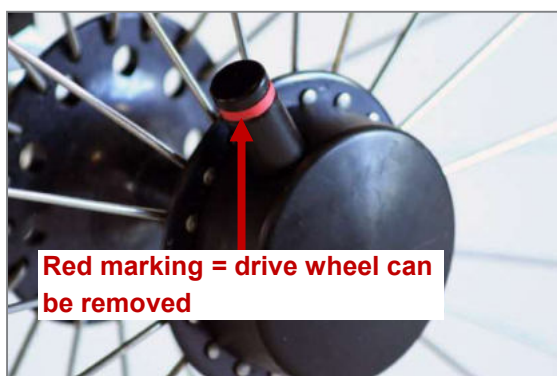
Figure 66: Tetra Clip with opened quick release axle, drive wheel can be removed
