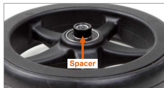
Figure 84: Spacer on the caster wheel
