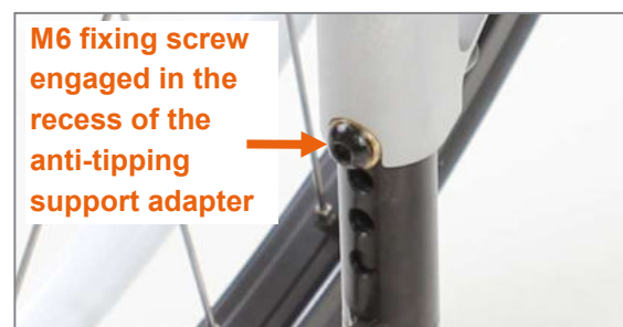
Figure 124: Anti-tipping support engaged correctly
