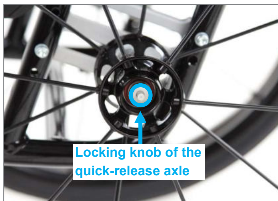
Figure 62: Locking knob of the quick-release axle in the middle of the wheel axle
