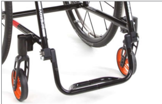
Figure 103: Footrest, fold up to the rear, in standard position
