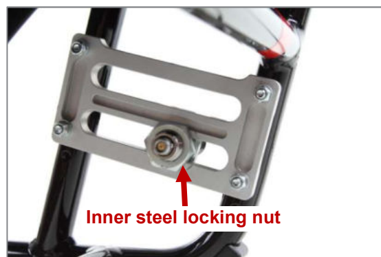
Figure 17: Inner steel locking nut (view from inside of product, drive wheel removed)
