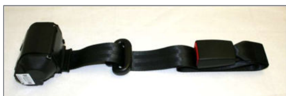
Figure 151: Automatic diagonal shoulder belt with deflector and buckle
