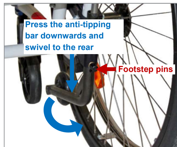
Figure 123: Moving the anti-tipping support to operating position (view from the rear)
