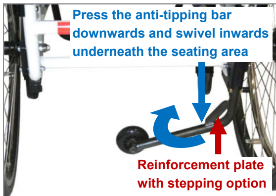
Figure 125: Moving the anti-tipping support to passive position (view from the rear)
