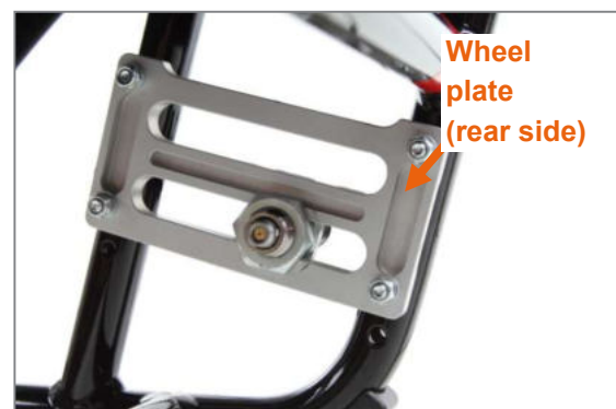
Figure 2: 2-slot wheel plate for rear seat height adjustment (view from inner side of product, drive wheel removed)
