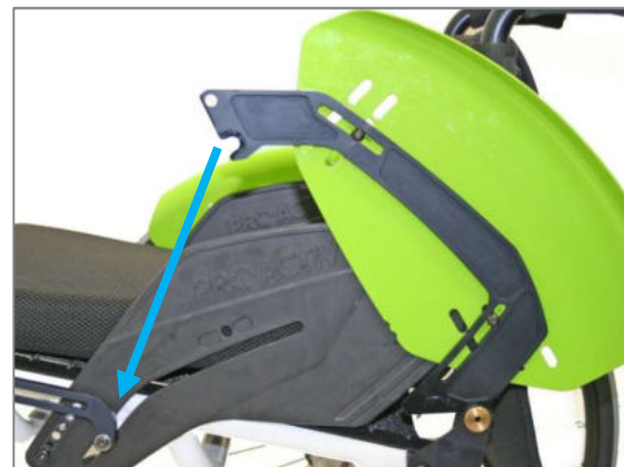
Figure 56: Mounting bar pinned on the back jointed shaft (shown without drive wheel)
