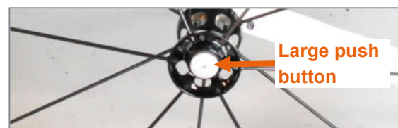
Figure 64: Quick-release axle with operation support, large push button
