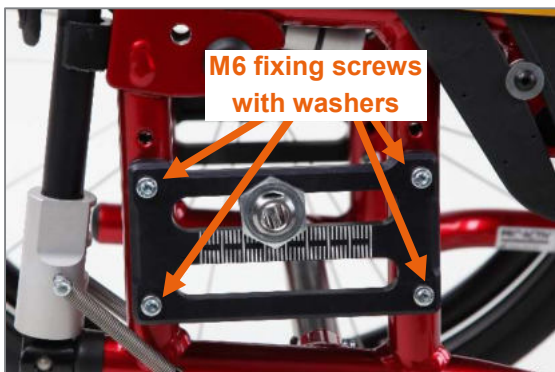
Figure 7: M6 fixing screws on the wheel plate (view from outer side of product, drive wheel removed)
