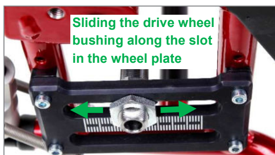
Figure 18: Sliding the drive wheel bushing along the slot in the wheel plate (view from outer side of product)
