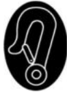
Figure 143: Karabiner symbol/sticker for a tested wheelchair approved for transporting passengers in motor vehicles
