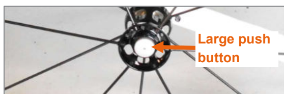
Figure 56: Quick-release axle with operation support, large push button
