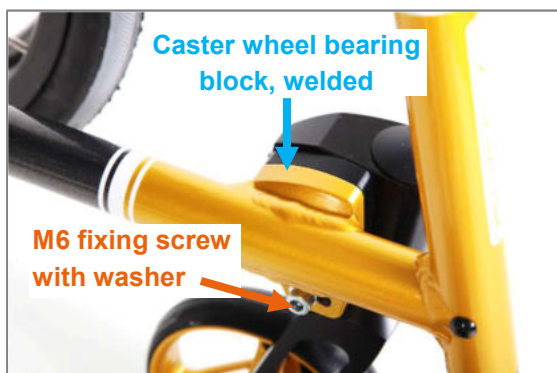
Figure 83: M6 fixing screw on the frame inner side with washer
