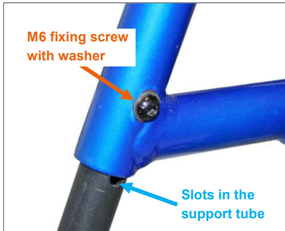
Figure 88: M6 fixing screw with washer and slot in footrest support tube for adjusting the lower leg length
