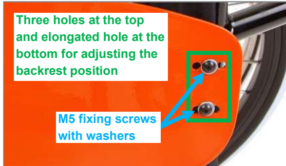
Figure 20: Adjusting the backrest position using holes in the side section
