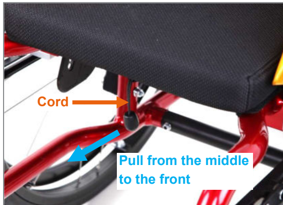
Figure 22: Cord for operating the locking pin and thus for adjusting the angle of the backrest
