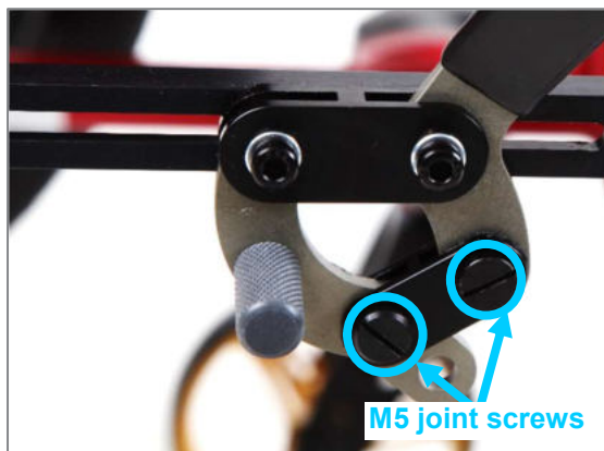
Figure 116: M5 joint screws for setting the actuating force of the brake lever
