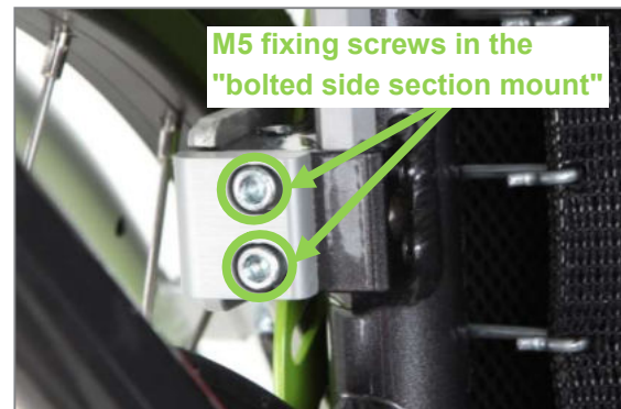
Figure 51: "Side section mount, bolted" with elongated holes and M5 fixing screws on basic body of side section mount (view from below)
