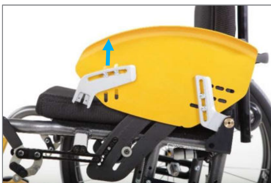
Figure 41: Clothing guard pulled from the "side section mount, bolted" at the front (view without drive wheel)
