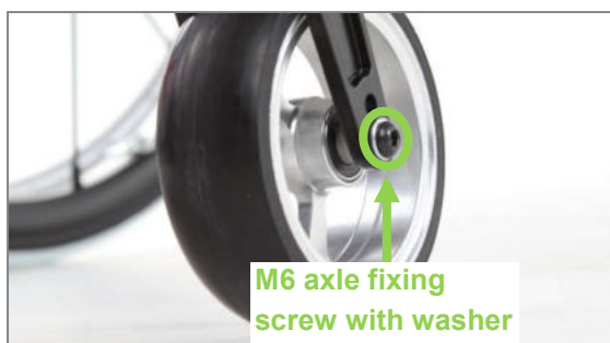
Figure 72: M6 axle fixing screw of caster wheel axle (view from outer side of product)
