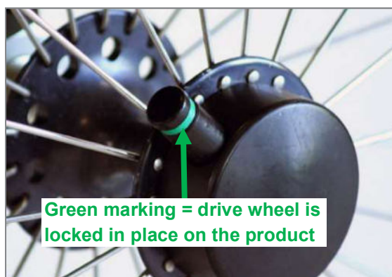
Figure 57: Tetra Clip with locked quick release axle
