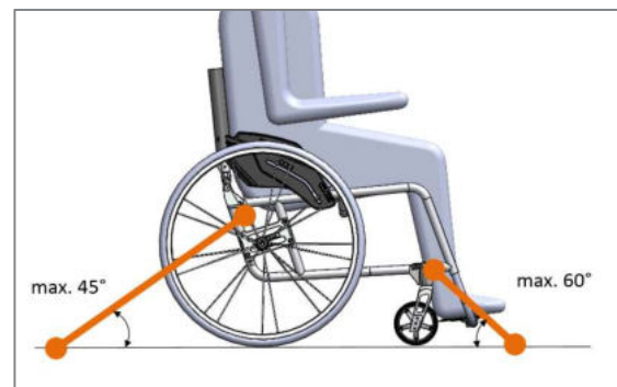
Figure 150: Run of the retractors at the front and rear with maximum tensioning angle and connecting points (view from the side)
