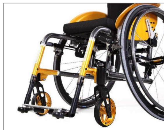
Figure 96: Footrest, folding up to the rear, with spring latching mechanism, in standard position
