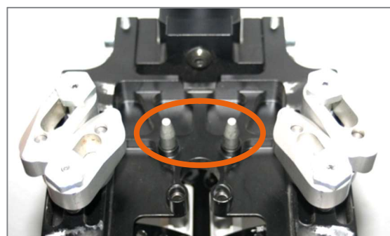
Figure 29: Centring pins assembled for wide centre part
