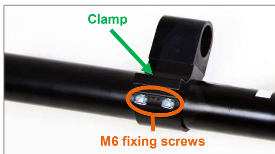
Figure 26: M6 fixing screws to horizontally position the centring column mount along the mounting tube
