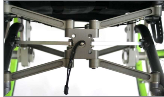
Figure 16: Release cord positioned incorrectly, drill holes for centring pins hidden to the bottom left
