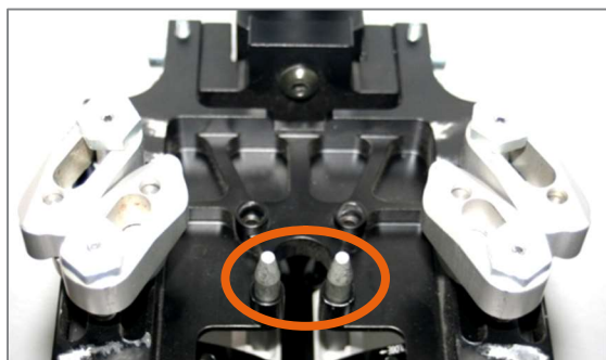
Figure 30: Centring pins assembled for narrow centre part
