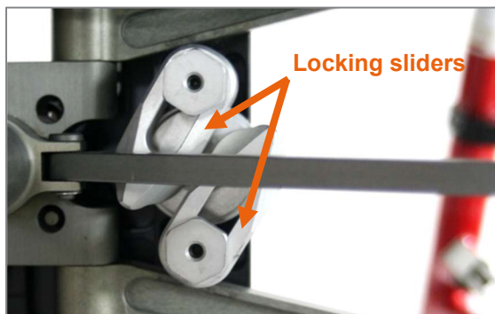
Figure 9: Back view of folding mechanism with open locking sliders
