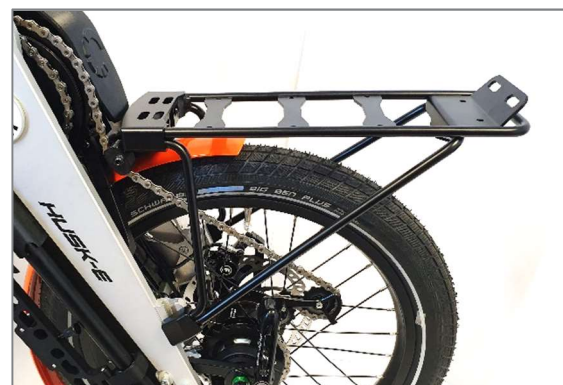
Figure 48: Luggage rack installed
