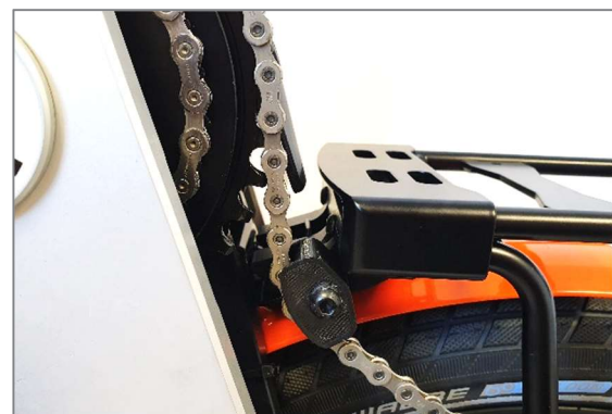
Figure 47: Luggage rack installed, chain deflector guide tensioning the chain
