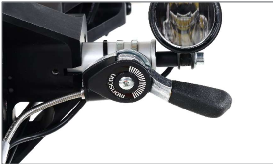
Figure 29: Parking brake via locking lever
