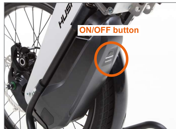
Figure 38: Switching the rechargeable battery on and off
