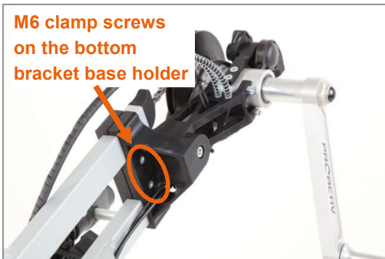
Figure 20: M6 clamp screws on the bottom bracket base holder for adjusting the length
