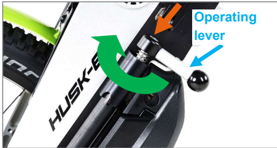
Figure 6: Press down and turn the operating lever
