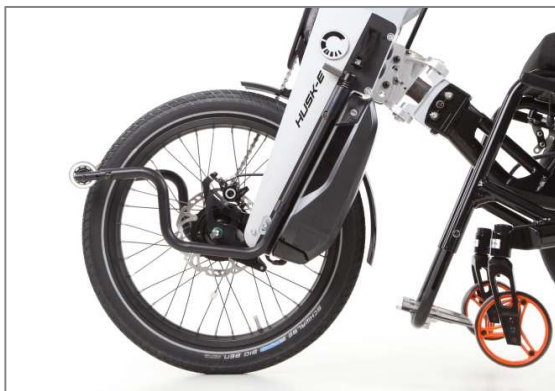
Figure 8: Parking stand in the passive position
