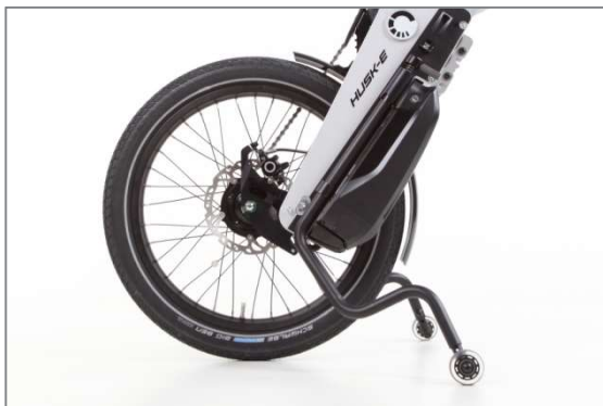
Figure 7: Parking stand in the active position
