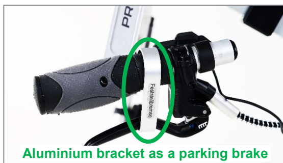
Figure 30: Aluminium bracket as a parking brake
