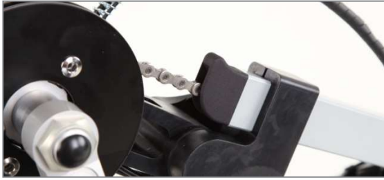
Figure 19: Plastic chain guides in rectangular tube
