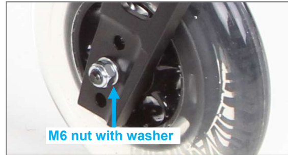
Figure 42: M6 caster wheel axle nut (view from inner side of product)
