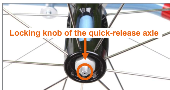
Figure 24: Locking knob of the quick-release axle in the middle of the wheel axle
