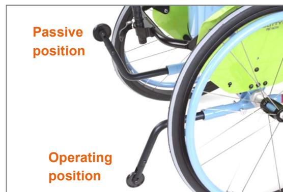
Figure 51: Operating and passive position of the anti-tippers
