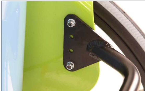
Figure 14: Connecting the back cross bar on the LITTY 4all
