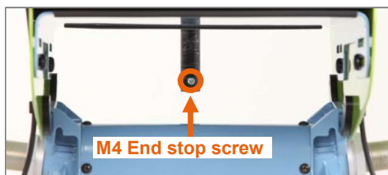
Figure 68: M4 end stop screw attached to bottom of central push handle
