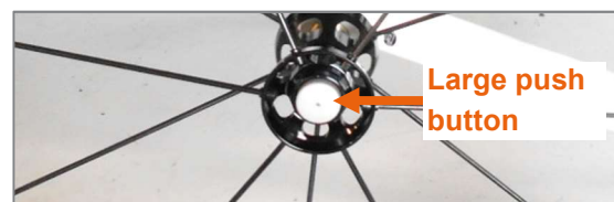
Figure 26: Quick-release axle with operation support, large push button
