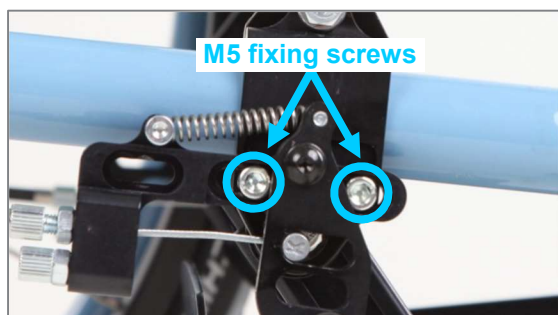
Figure 61: M5 fixing screws
