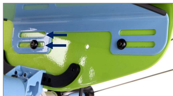
Figure 8: Seat plate slots at different heights
