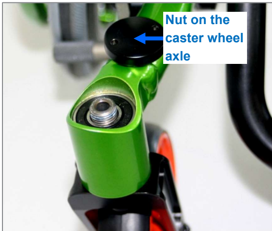
Figure 47: Caster wheel axle nut completely removed
