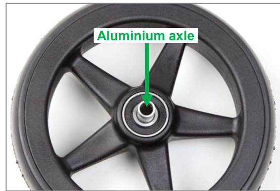
Figure 43: Caster wheel with aluminium axle
