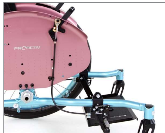
Figure 60: Knee lever brake with brake operation integrated in the clothing guard
