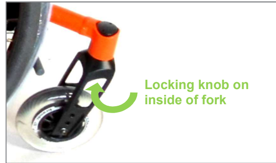
Figure 48: Caster wheel fork with quick release axle and locking knob
