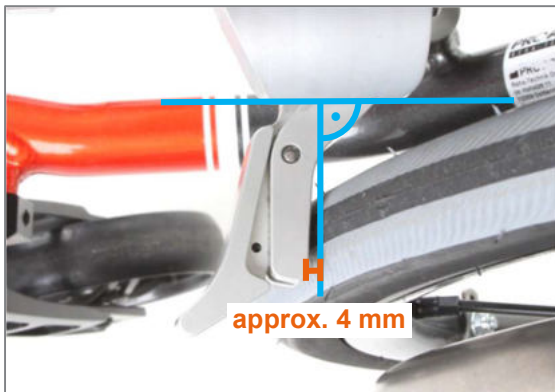
Figure 157: Brake element after correct positioning of the integral brake
