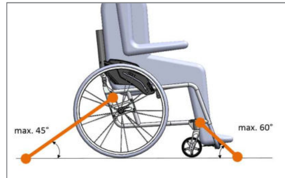
Figure 184: Run of the retractors at the front and rear with maximum tensioning angle and connecting points (view from the side)
