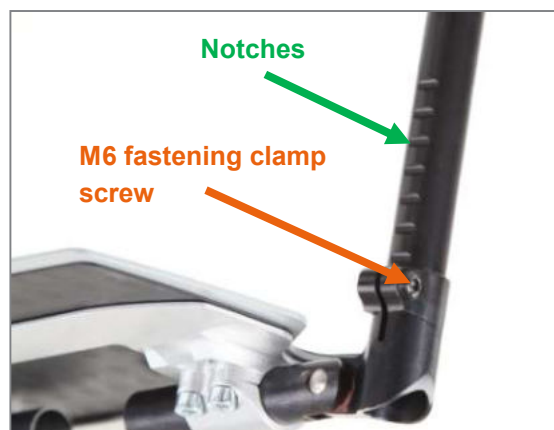
Figure 119: Notches and M6 fastening clamp screw for lower leg length adjustment (view from the rear)
