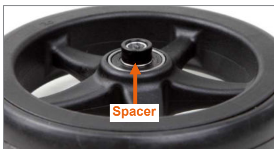
Figure 93: Spacer on the castor wheel
