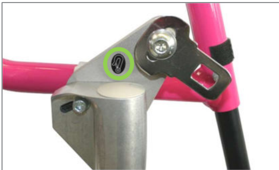
Figure 178: Caster wheel bearing block intermediate plate with belt link for mounting the front retractor
