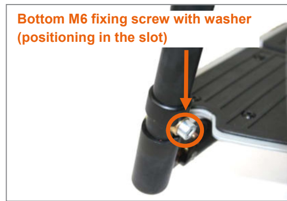
Figure 123: Bottom M6 fixing screw (AF 5 mm) can be positioned in the slot
