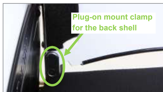
Figure 48: Plug-on mount clamp for the back shell (view from front)
