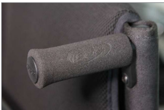
Figure 164: Push handles, horizontally screwed in back tube
