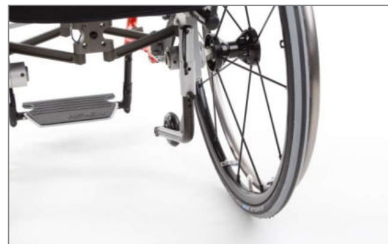
Figure 131: Passive position of anti-tipping support (view from the rear)
