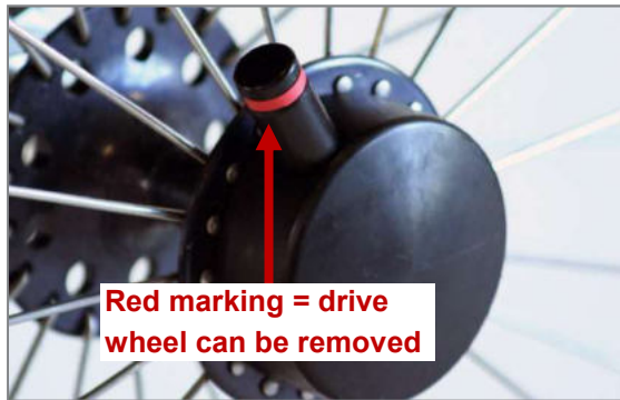
Figure 71: Tetra Clip with opened quick release axle, drive wheel can be removed
