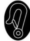
Figure 175: Karabiner symbol/sticker for a tested wheelchair approved for transporting passengers in motor vehicles
