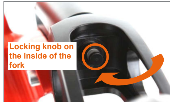
Figure 98: Caster fork with quick-release axle and locking knob
