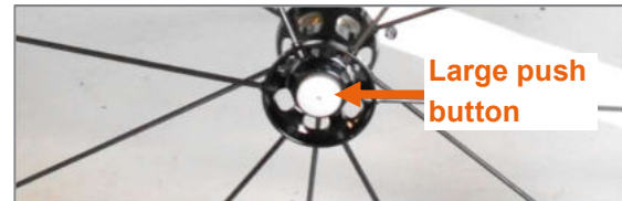
Figure 69: Quick-release axle with operation support, large push button
