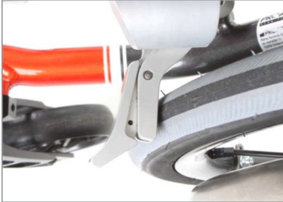
Figure 156: Brake element resting on the tyre
