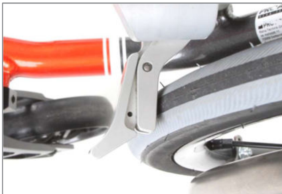
Figure 160: Brake element resting on the tyre
