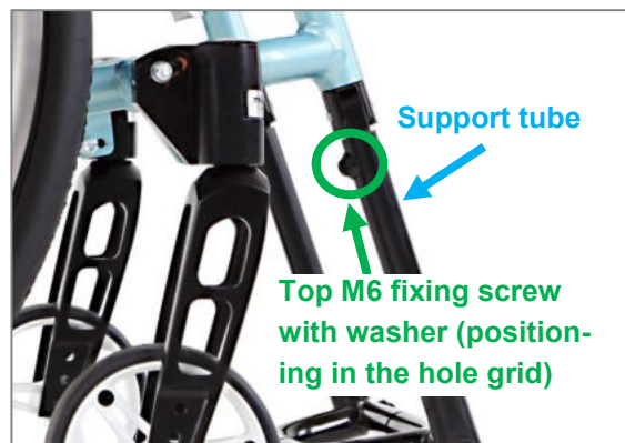
Figure 108: Top M6 fixing screw can be positioned in the hole grid
