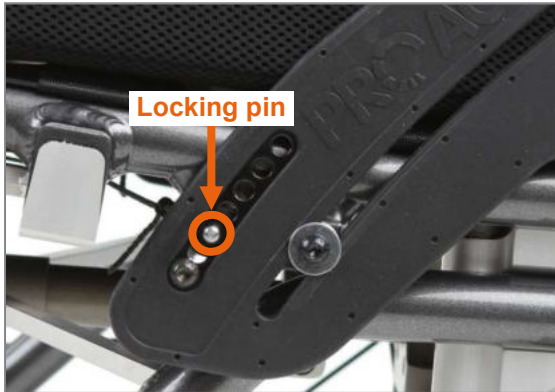
Figure 24: Locking pin engages in the locking hole in the side section (view from outer side of product, without clothing guard)
