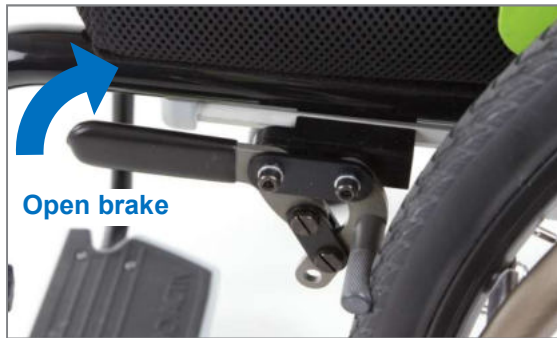
Figure 145: Brake closed; to open, pull the brake lever up and rearwards
