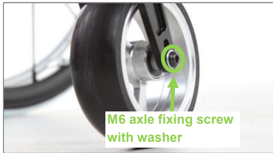
Figure 90: M6 axle fixing screw of castor wheel axle (view from outer side of product)
