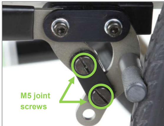
Figure 148: M5 joint screws for setting the actuating force of the brake lever
