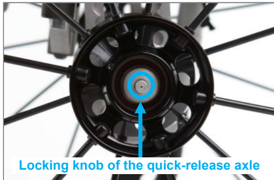
Figure 67: Locking knob of the quick-release axle in the middle of the wheel axle
