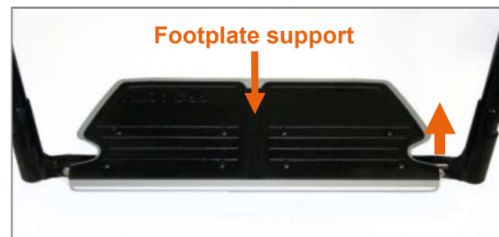
Figure 111: For folding up to one side, lift the footrest up in the direction of travel on the left side (product view from the front)
