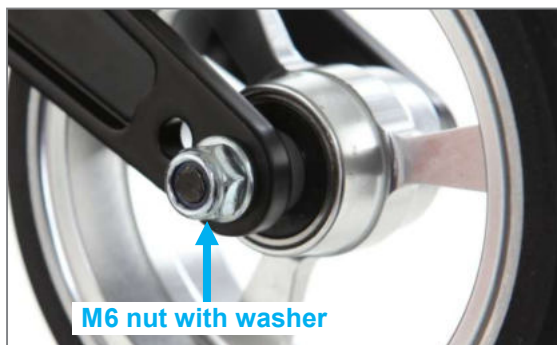
Figure 91: M6 castor wheel axle nut (view from inner side of product)
