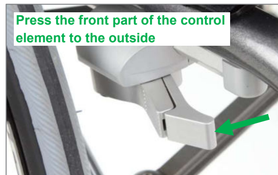
Figure 151: Integral brake open, closing is carried out by pressing the control element outwards
