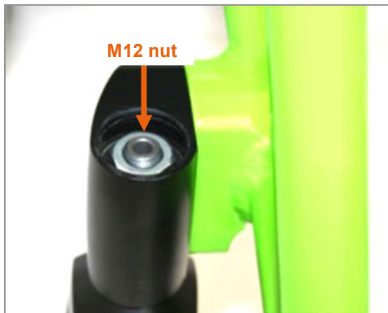
Figure 97: Aluminium cap removed and M12 nut visible
