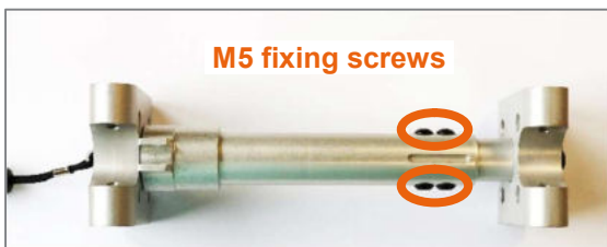
Figure 21: M5 fixing screws of the folding mechanism middle section (the folding mechanism middle section is shown as a separate part for better illustration, side view)
