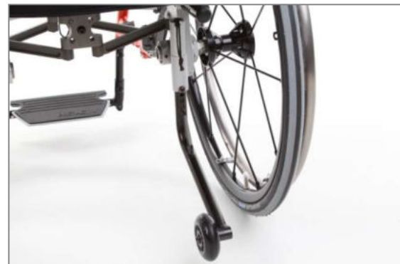
Figure 130: Operating position of anti-tipping support (view from the rear)
