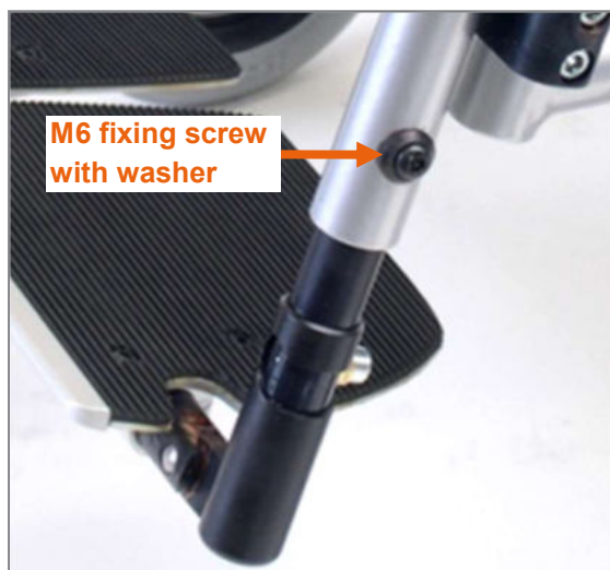
Figure 122: M6 fixing screw with washer to adjust the lower leg length
