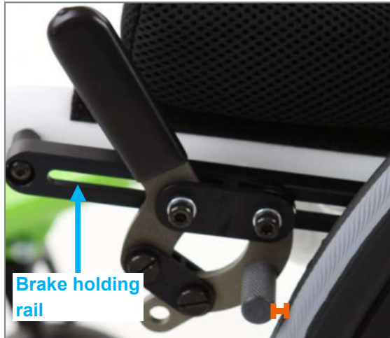
Figure 138: Distance between the brake pin and tyre of approx. 3 to max. 4 mm with the brake opened
