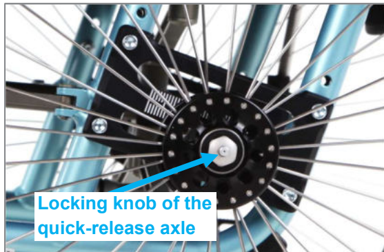
Figure 66: Locking knob of the quick-release axle in the middle of the wheel axle
