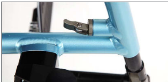
Figure 99: Locking bolt lever released or set perpendicular to the holder to remove the footrest
