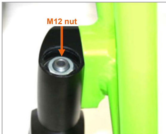
Figure 91: Aluminium cap removed and M12 nut visible
