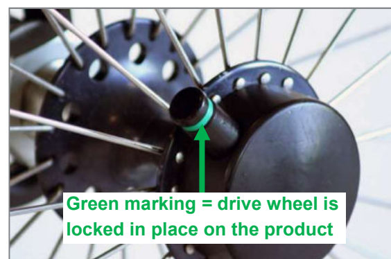
Figure 69: Tetra Clip with locked quick release axle
