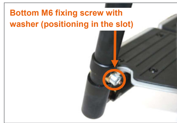
Figure 117: Bottom M6 fixing screw (AF 5 mm) can be positioned in the slot
