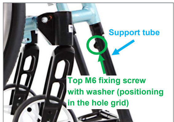
Figure 102: Top M6 fixing screw can be positioned in the hole grid
