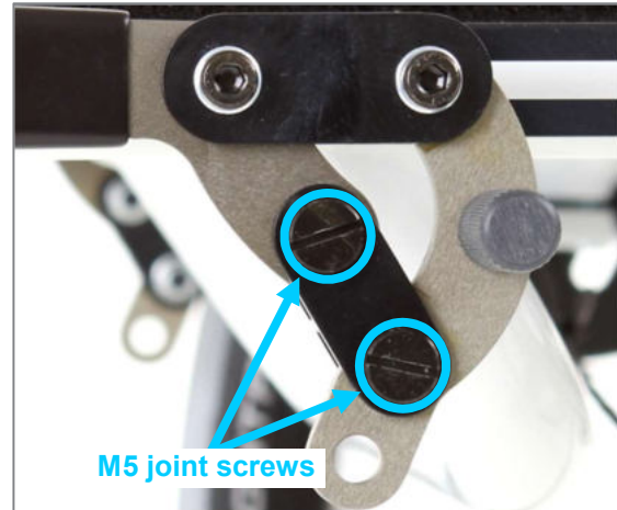
Figure 139: M5 joint screws for setting the actuating force of the brake lever
