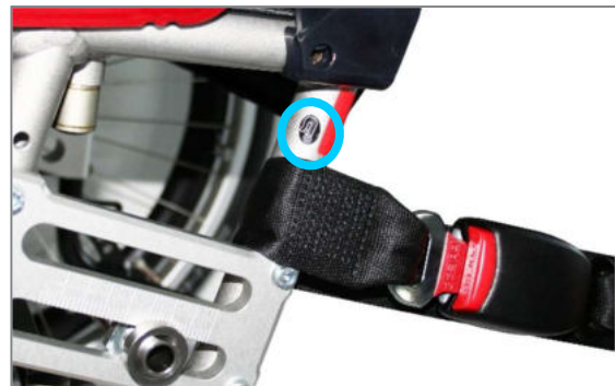
Figure 162: Symbol for rear fastening and wheelchair loop at the rear
