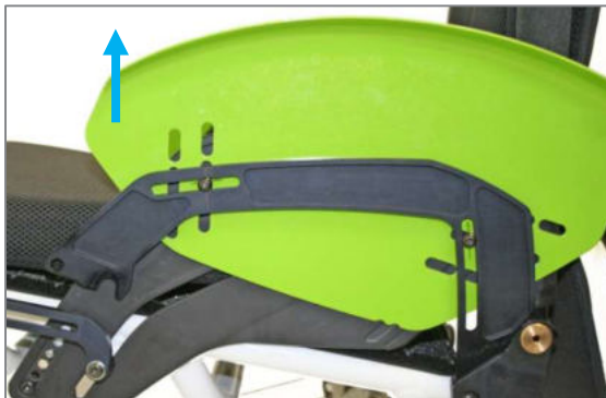
Figure 59: Clothing guard pulled from the side panel guide to the front (shown without drive wheel)
