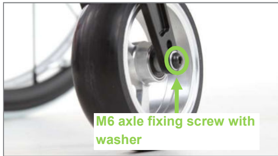
Figure 84: M6 axle fixing screw of caster wheel axle (view from outer side of product)
