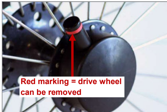
Figure 70: Tetra Clip with opened quick release axle, drive wheel can be removed
