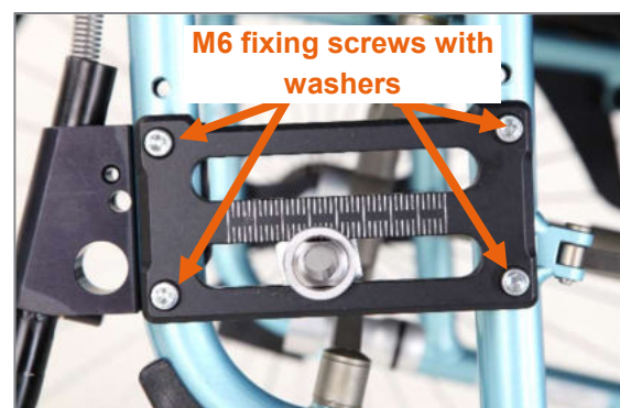
Figure 12: M6 fixing screws on the wheel plate (view from outer side of product, drive wheel removed)
