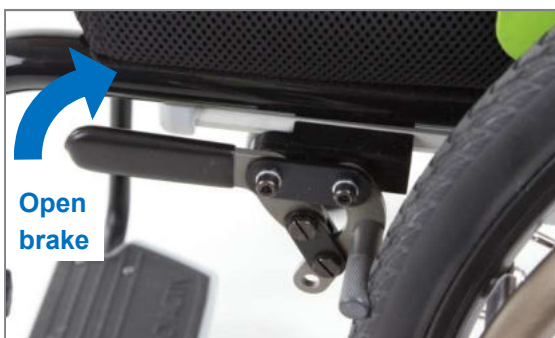
Figure 136: Brake closed; to open, pull the brake lever up and rearwards
