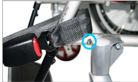
Figure 161: Symbol for front fastening and wheelchair loop at the front
