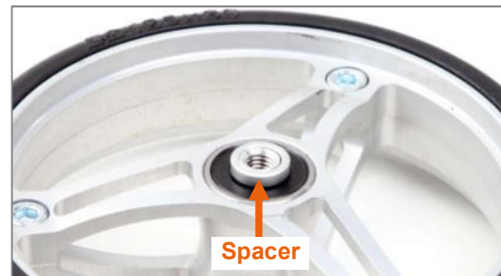
Figure 83: Spacer on the caster wheel
