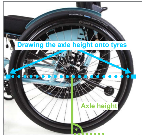
Figure 72: Drawing the axle height on the front and back of both tyres
