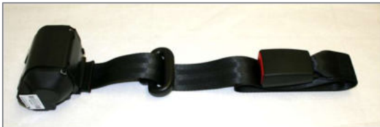
Figure 154: Automatic diagonal shoulder belt with deflector and buckle
