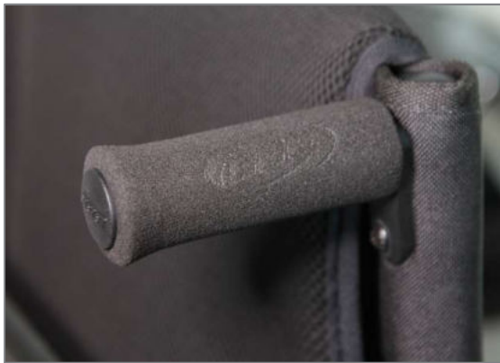
Figure 145: Push handles, horizontally screwed in back tube
