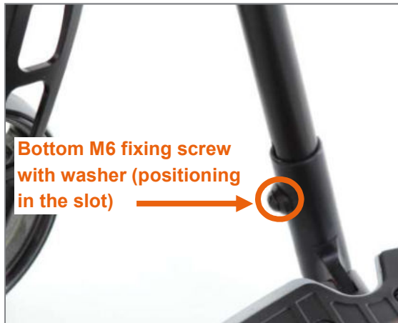
Figure 103: Bottom M6 fixing screw can be positioned in the slot
