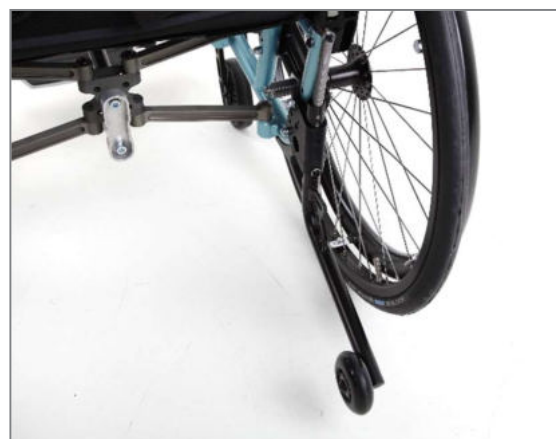
Figure 124: Operating position of anti-tipping support (view from the rear)
