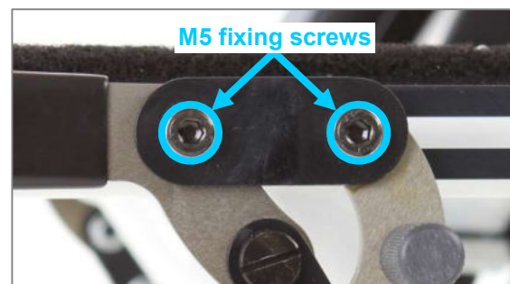
Figure 137: M5 fixing screws on the brake holding rail
