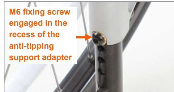
Figure 127: Anti-tipping support engaged correctly
