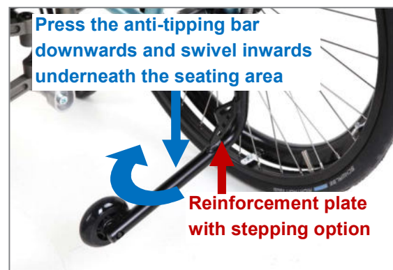
Figure 128: Moving the anti-tipping support to passive position (view from the rear)
