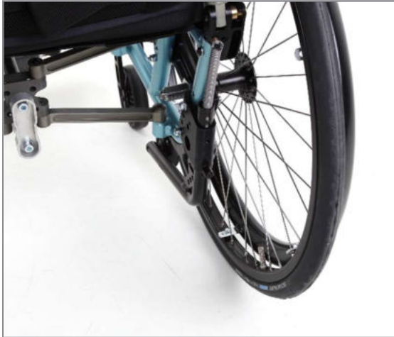
Figure 125: Passive position of anti-tipping support (view from the rear)
