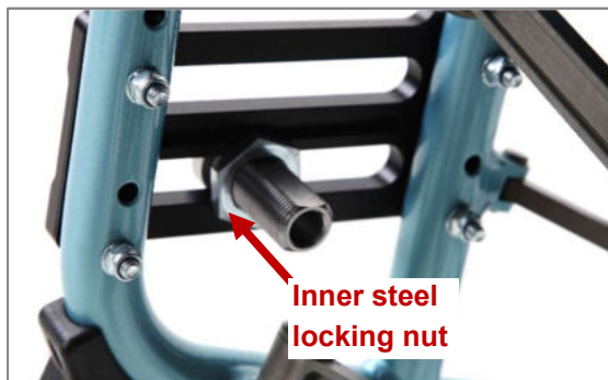
Figure 10: Inner steel locking nut (view from inside of product, drive wheel removed)
