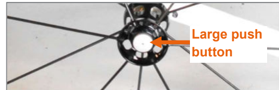
Figure 68: Quick-release axle with operation support, large push button
