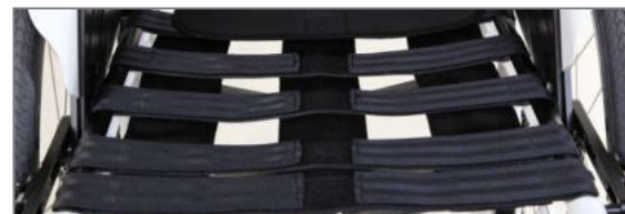
Figure 51: Open belt system with fleece hook-and-loop straps for adjusting the slack
