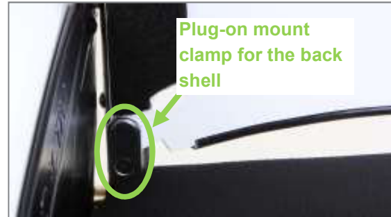
Figure 50: Plug-on mount clamp for the back shell (view from front)
