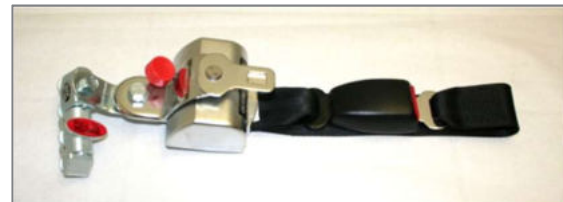
Figure 151: Front retractor "semi-automatic" with buckle and belt link
