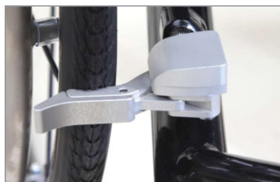
Figure 163: Fixing the integrated brake to the lower frame tube
