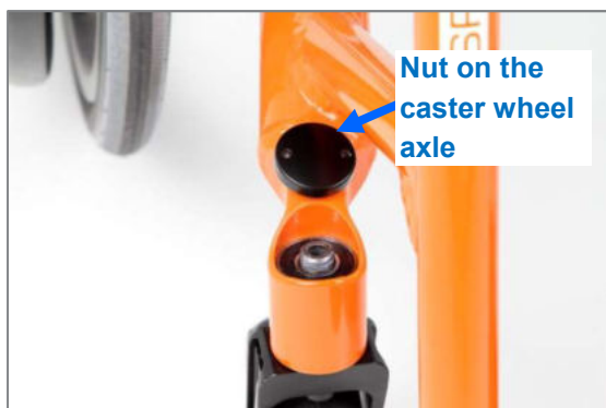
Figure 94: Caster wheel axle nut completely removed
