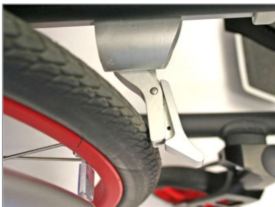
Figure 159: Brake element resting on the tyre
