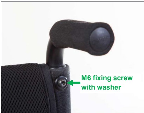
Figure 169: Aluminium push handles fixed in back tube
