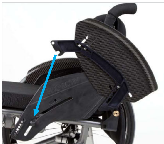
Figure 48: Mounting bar pinned on the back jointed shaft (shown without drive wheel)
