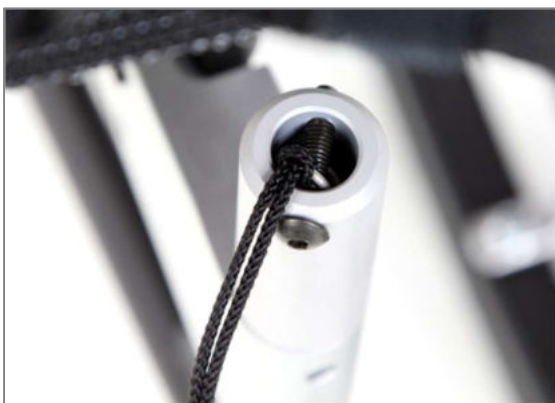
Figure 128: The M5 fixing screw screwed through the end eyelets of the tension spring
