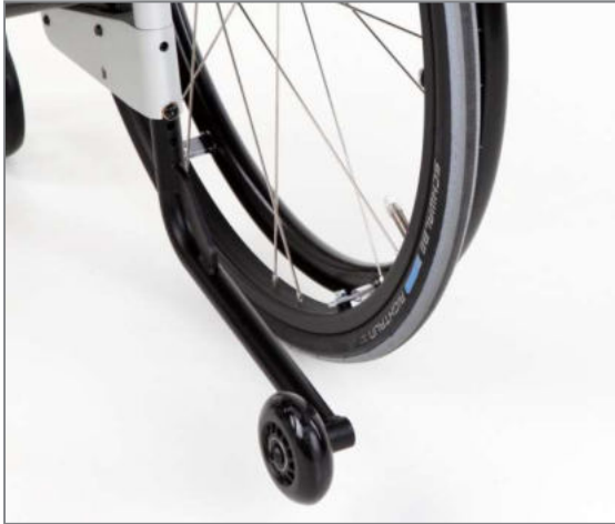
Figure 119: Operating position of anti-tipping support (view from the rear)
