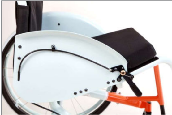
Figure 144: Knee lever brake with pull cable operation, control unit
