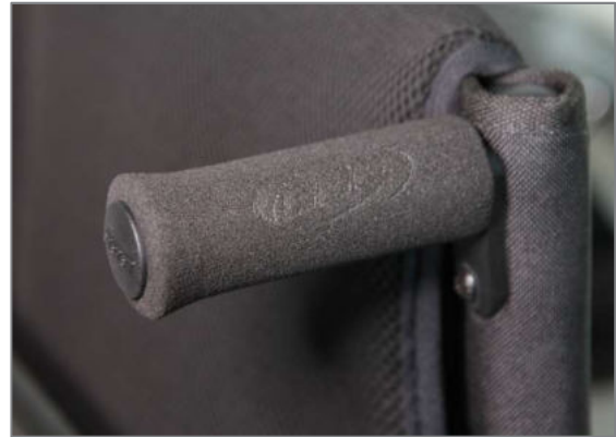
Figure 170: Push handles, horizontally screwed in back tube
