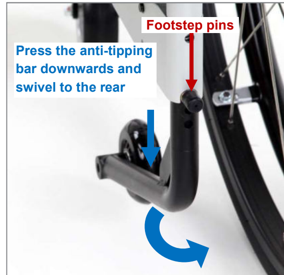
Figure 121: Moving the anti-tipping support to operating position (view from the rear)
