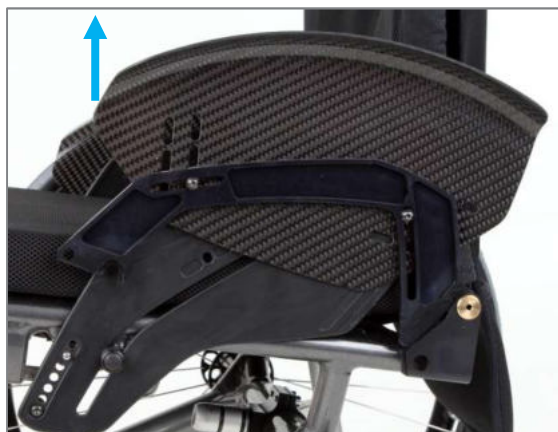
Figure 47: Clothing guard pulled from the side panel guide to the front (shown without drive wheel)
