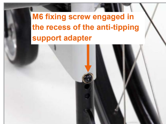
Figure 122: Anti-tipping support engaged correctly
