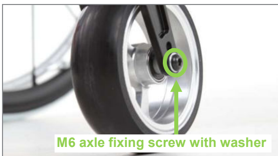
Figure 85: M6 axle fixing screw of caster wheel axle (view from outer side of product)
