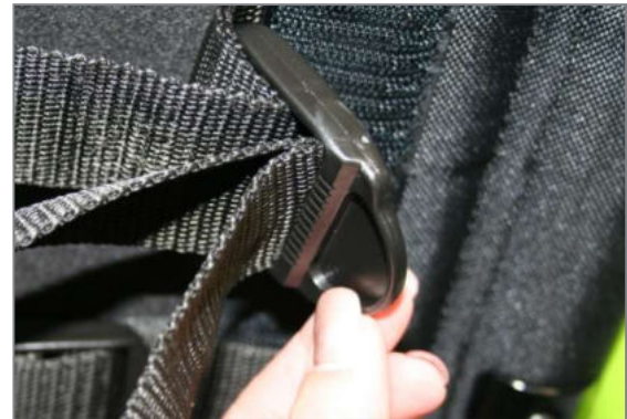
Figure 22: Step 5: Returning the belt through the tensioning loop to obtain the required "double passage"
