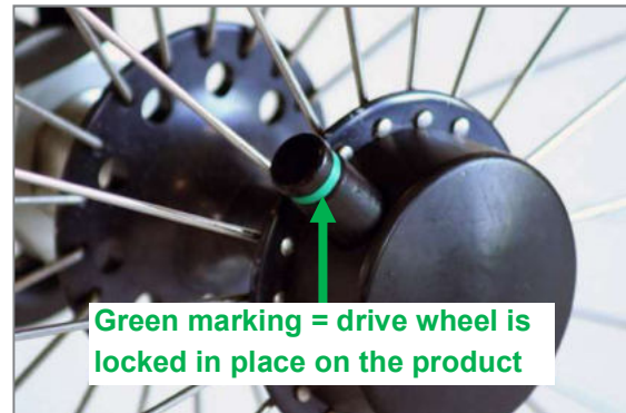
Figure 57: Tetra Clip with locked quick release axle
