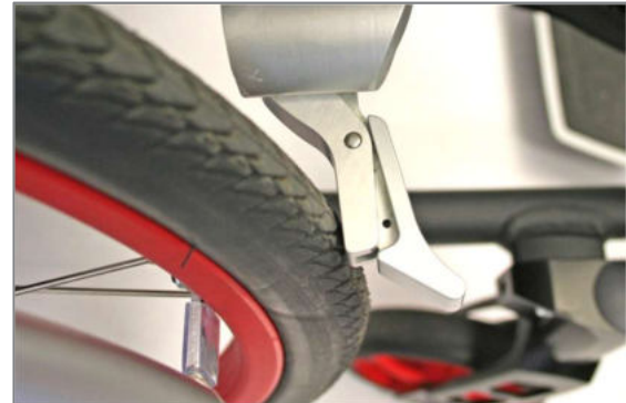
Figure 166: Brake element resting on the tyre
