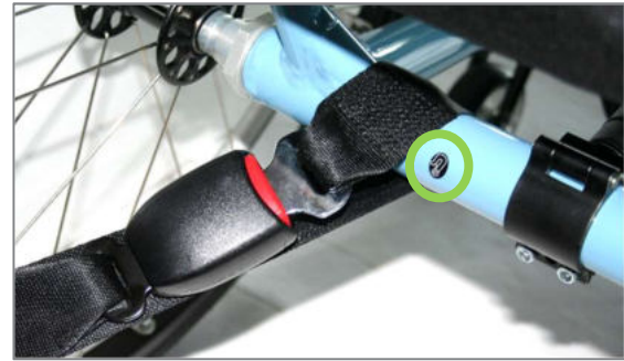
Figure 183: Symbol for rear fastening and wheelchair loop at the rear
