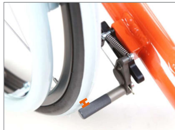
Figure 151: Distance between brake pin and tyre of approx. 3 mm to maximum 4 mm, with opened brake
