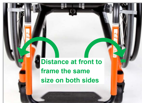
Figure 63: Front distance to the frame (SPEEDY F2 oversized)
