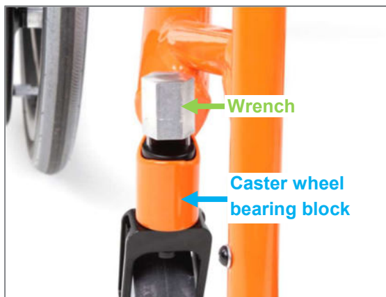
Figure 93: Loosen the nut of the caster wheel axle using the wrench
