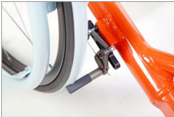
Figure 145: Knee lever brake with pull cable operation, braking unit
