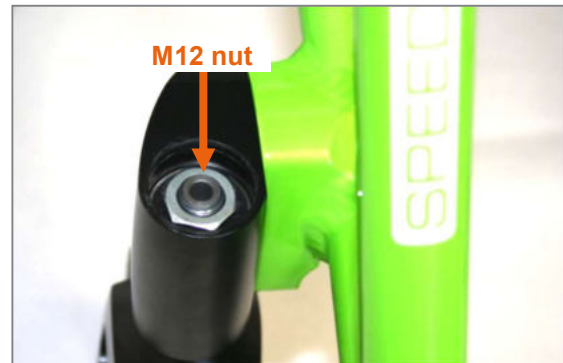
Figure 92: Aluminium cap removed and M12 nut visible
