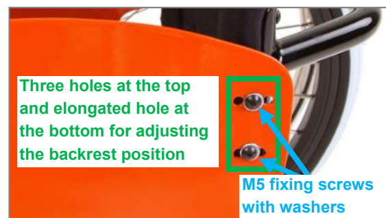
Figure 5: Adjusting the backrest position using holes in the side panel or the clothing guard
