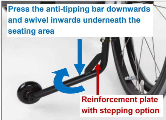
Figure 123: Moving the anti-tipping support to passive position (view from the rear)
