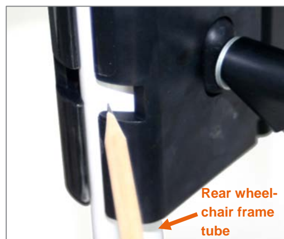
Figure 52: Drawing the position of the clamp frame stopper on the back of the wheelchair's frame tube
