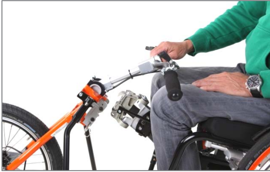
Figure 79: Inserting the insertion bolt of the docking plate in the insertion shaft on the steering head
