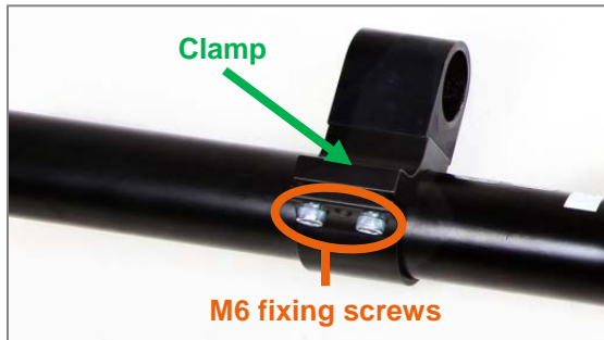
Figure 9: M6 positioning screws to horizontally position the centring column mount
