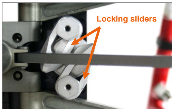
Figure 13: Back view of folding mechanism with open locking sliders
