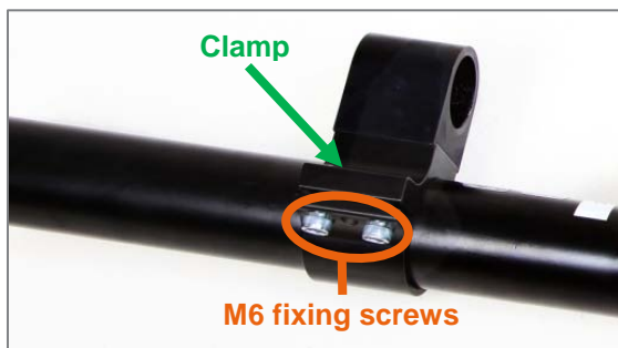
Figure 29: M6 fixing screws to horizontally position the centring column mount along the adapter tube
