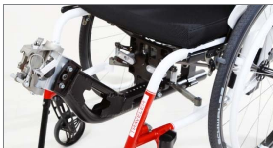
Figure 1: Central adapter on folding mechanism
