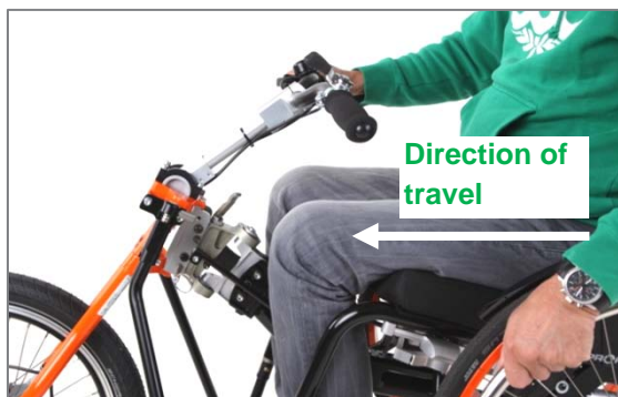
Figure 85: Press the product's brake and move towards the product with the grip rings until it unlocks
