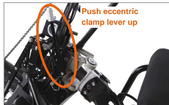
Figure 67: Eccentric clamp lever is pushed to "clamp"
