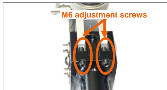
Figure 22: M6 setting screws resting on the steering head connection
