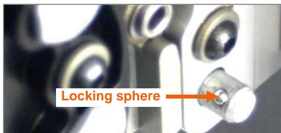
Figure 69: Securing bolt with locking sphere, locking sphere locked on the right outer side of the docking plate
