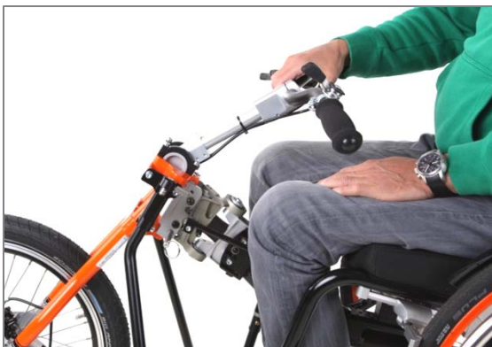
Figure 80: Insertion bolt inserted into the insertion shaft on the steering head
