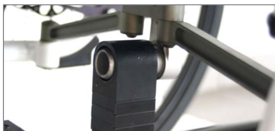
Figure 14: Centring column with inserted holder
