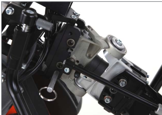
Figure 91: Adapter head completely positioned on the docking plate
