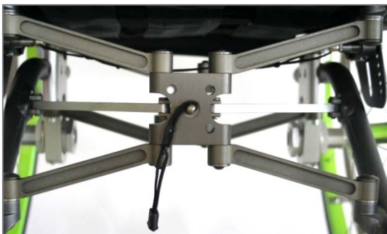
Figure 18: Release cord positioned incorrectly, drill holes for centring pins hidden to the bottom left
