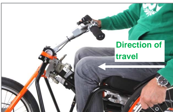
Figure 81: Press the product's brake and move towards the product with the grip rings until it clicks into place
