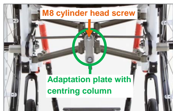
Figure 3: Folding mechanism with adaptation plate and centring column (wheelchair from behind)
