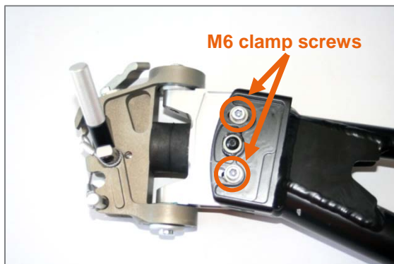
Figure 20: M6 clamp screws on steering head
