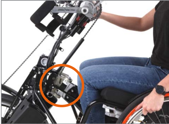
Figure 64: Inserting the insertion bolt of the docking plate in the insertion shaft on the steering head
