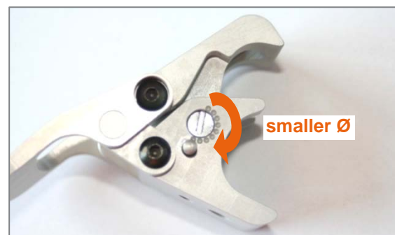
Figure 40: Turning the eccentric shaft along the marking points (clockwise for smaller Ø, anti-clockwise for larger Ø)
